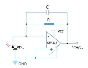
$$\begin{split} &V_{out}(V) = I_{ph}(A) \times R(\Omega) \\ &I_{ph}(A) = R_{\lambda}(A/W) \times A(cm^2) \times P(W/cm^2) \\ &\text{where A is chip area.} &\text{$\Psi$ is implicated in $UV$ power denisity} \\ &\text{and $R_{\lambda}$ is responsivity at specific wavelength.} \end{split}$$
